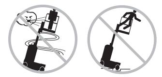
Do not drive the machine on or near uneven terrain, unstable surfaces or other hazardous conditions with the platform raised. Do not replace items critical to machine stability with items of different weight or specification.
