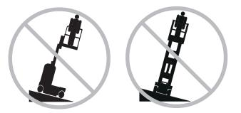
Do not depend on the tilt alarm as a level indicator. The tilt alarm sounds only when the machine is on a slope.
